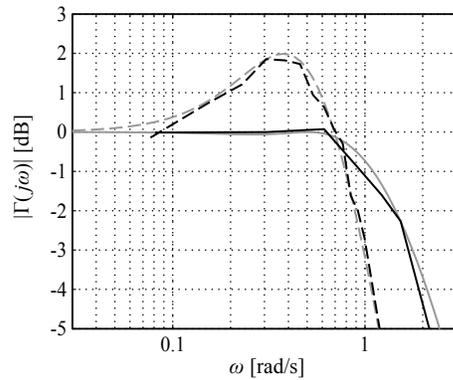
Fig. 9. String stability complementary sensitivity  $|\Gamma(j\omega)|$ : (solid grey) CACC, simulated, (solid black) CACC, measured, (dashed grey) ACC, simulated, (dashed black) ACC, measured.
