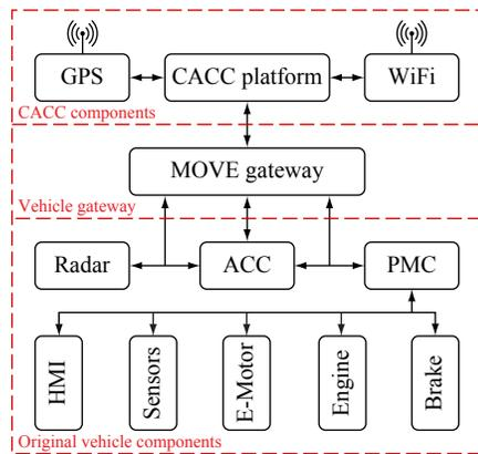
Fig. 5. Schematic representation of the test vehicle instrumentation.
