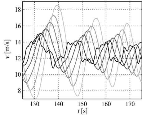
Fig. 7. Measured ACC velocity response: (black–light grey) vehicle 1–6.
