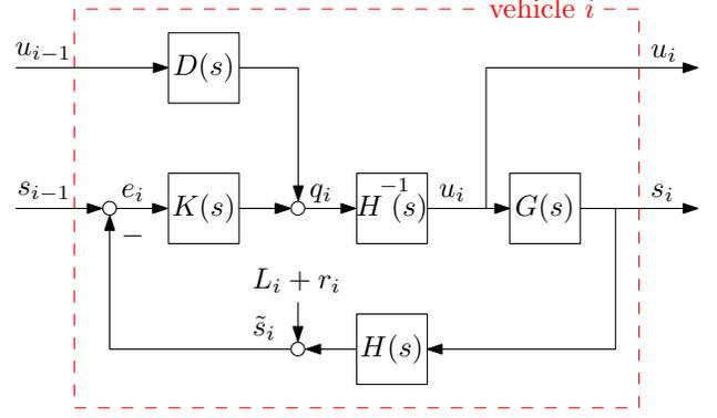
Fig. 3. Block scheme of the CACC system.
