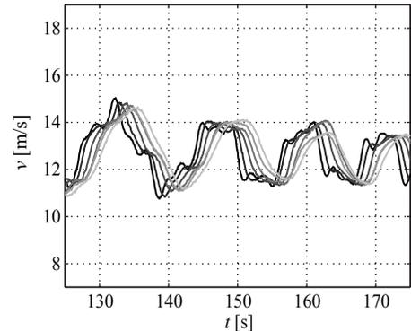
Fig. 8. Measured CACC velocity response: (black–light grey) vehicle 1–6.
