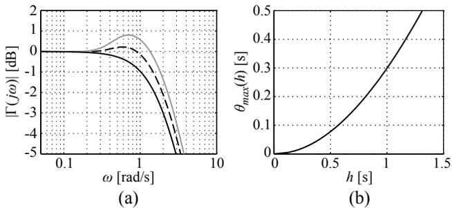
Fig. 4. String stability properties: (a) string stability complementary sensitivity  $|\Gamma(j\omega)|$  for communication delay (solid black)  $\theta = 0$  s, (dashed black)  $\theta = 0.15$  s, and (solid grey)  $\theta = 0.3$  s, and (b) maximum string stable communication delay  $\theta_{max}(h)$ .
