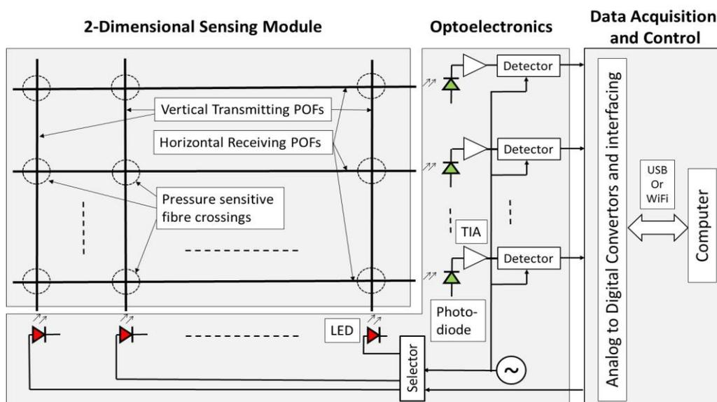
Figure 1. 2D position sensing system deploying a matrix of step index plastic optical fibre (SI-POF) crosspoints.
