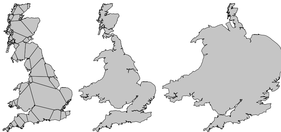
Fig. 6. (left) A polygon representing Great Britain with the edges of a MINSIZEPOLY solution with \tau = 2 . Variable-scale maps computed (middle) without and (right) with consideration of the selected diagonals. The method of Haunert and Sering [11] was used with a scale factor of 2 for Wales; the results were scaled to the same height.
