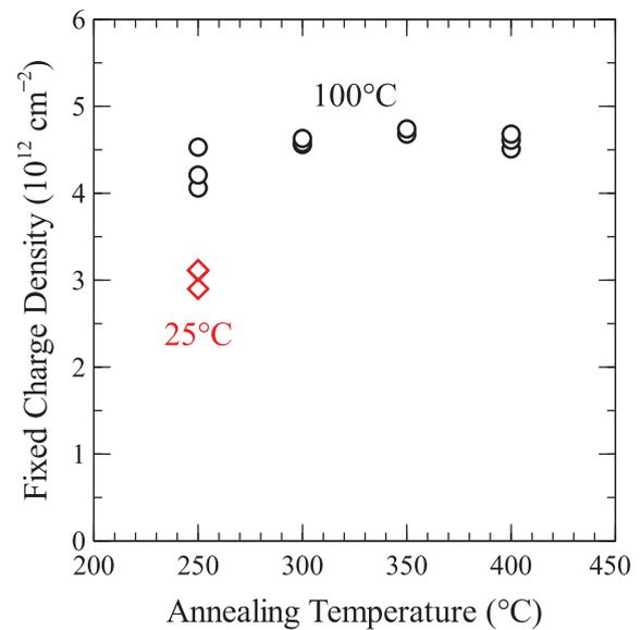
Fig. 8. Fixed charge density determined by high-frequency capacitance–voltage measurements for  $\text{PO}_x/\text{Al}_2\text{O}_3$  stacks deposited on  $n$ -type silicon at 100 °C and 25 °C as a function of annealing temperature (annealing was performed prior to metallisation for 10 min in  $\text{N}_2$ ).
