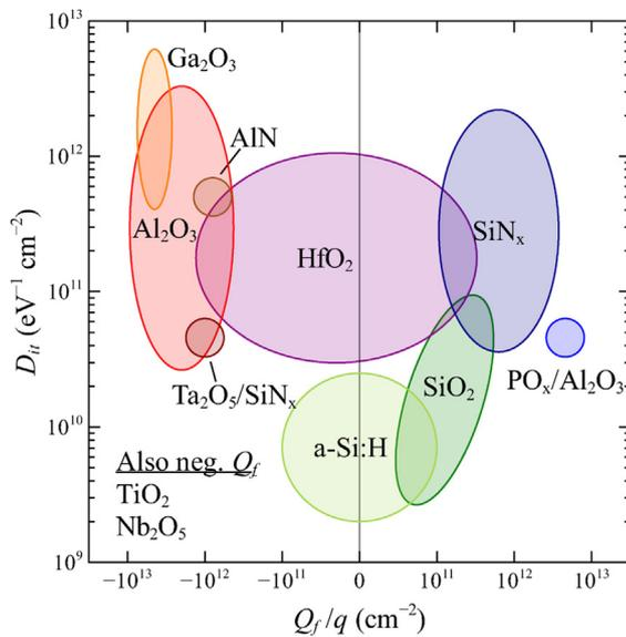
**Fig. 9.** Schematic comparison of different c-Si surface passivation materials and stacks in terms of interface state density  $D_{it}$  and fixed charge  $Q_f$ . Adapted with modifications from Cuevas et al. [17]. The approximate position of  $PO_x/Al_2O_3$  is indicated. Additional passivation materials for which the charge polarity is known to be negative, but for which the magnitude of both  $D_{it}$  and  $Q_f$  has not been reported ( $TiO_2$  [5],  $Nb_2O_5$  [8]), are noted.
