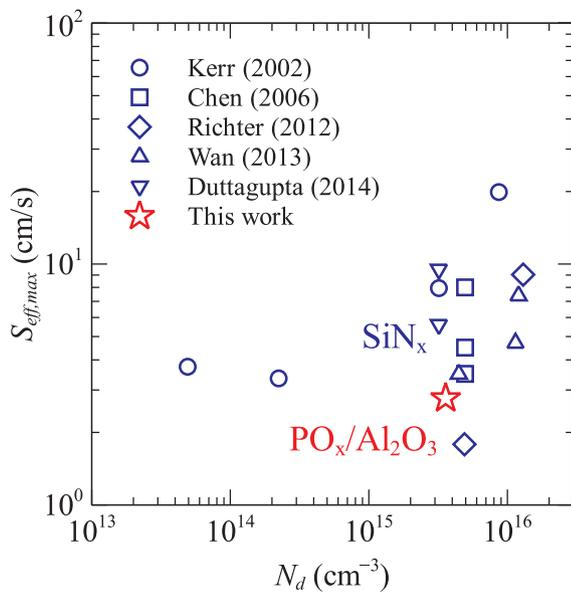
**Fig. 10.** Summary of  $S_{eff,max}$  at  $\Delta n = 10^{15} \text{ cm}^{-3}$  reported in the literature [14,21–25] as exemplary values for PECVD  $SiN_x$ , on  $n$ -type silicon as a function of dopant concentration  $N_d$ . Our best result for  $PO_x/Al_2O_3$  (deposited at  $100^\circ\text{C}$  and annealed up to  $450^\circ\text{C}$  in  $N_2$ ) is included for comparison.
