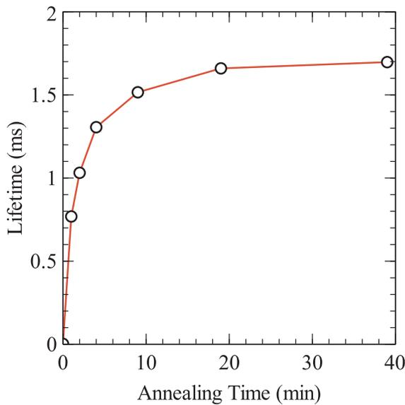
Fig. 7. Excess carrier lifetime  $\tau_{eff}$  ( $\Delta n = 10^{15} \text{ cm}^{-3}$ ) as a function of cumulative annealing time at 300 °C in  $\text{N}_2$  for an  $n$ -type Si (100) wafer passivated by  $\text{PO}_x/\text{Al}_2\text{O}_3$  deposited at 100 °C.
