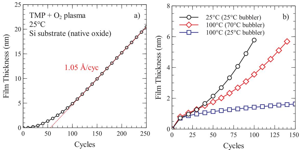
**Fig. 1.** Film thickness vs number of deposition cycles for PO<sub>x</sub> films deposited a) at 25 °C on a polished (100) Si substrate with a native oxide (25 °C bubbler temperature), and b) at 25 or 100 °C on HF-etched, polished (100) Si substrates (for bubbler temperatures of 25 °C and 70 °C). The TMP dose time was 500 ms in all cases (with a 10 s hold step).
