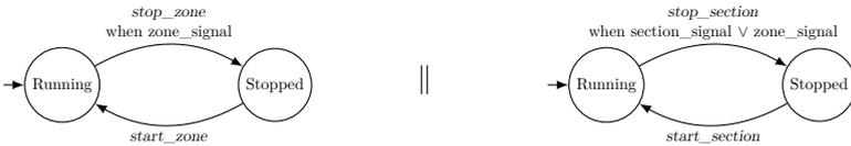
Figure 2.3: Duplication of guards when synchronization is not allowed.
