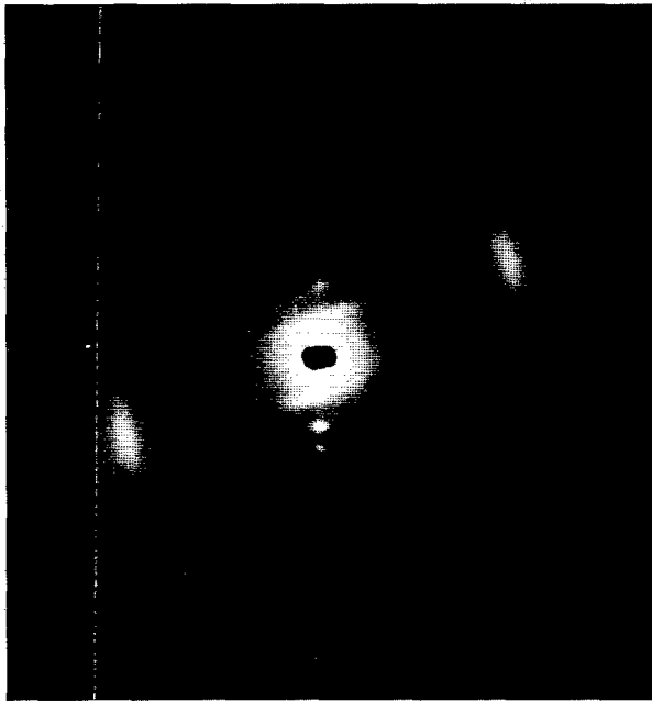
FIG. 9. X-ray diffraction photo of the anisotropic network.
