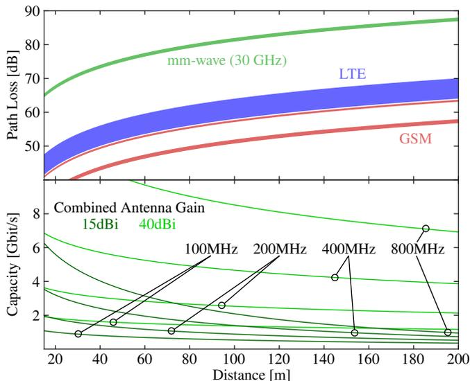
Figure 1. (a) Comparison of path loss between the traditional RF bands and the mm-wave band; (b) Achievable capacity at mm-wave frequencies for different bandwidths and antenna gains.
