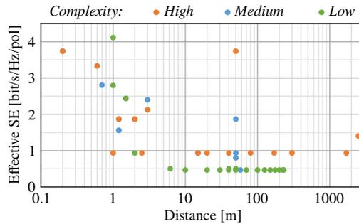
Figure 2. Spectral efficiency over distance for recent experimental demonstrations of point-to-point mm-wave links, classified by their implementation complexity; the points at 50 m and spectral efficiency larger 1.7 bit/s/Hz and 3.5 bit/s/Hz respectively stem from [10] and [12].
