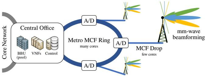
Figure 3. Overview of the *blueSPACE* radio access network architecture, based on analog radio-over-fiber fronthaul, space division multiplexing using multi-core fiber and mm-wave beamforming. BBU: base band unit, VNFs: virtualized network functions, MCF: multi-core fiber, A/D: multi-core add/drop multiplexer.
