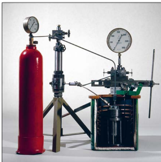
◀ FIG. 4: Apparatus used by Fawcett and Gibson in the discovery of polyethene in 1933. Next to the ethene feed are a primary gas compressor, the reactor vessel (filled with oil, a mercury interphase, and liquid benzaldehyde) and the oil press for reaching up to 3000 atm. [© Science Museum, London]
