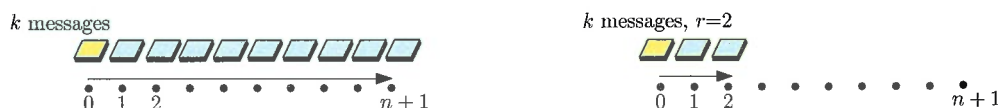
Figure 1: Illustration of the scenarios. Left: with unbounded reach, the k messages arrive immediately to all nodes, but that does not prevent intermediate nodes from forwarding the messages. Right: with range r = 2 , the messages sent from node 0 only reach up to node 2, so forwards are necessary to reach the target, n + 1 .
