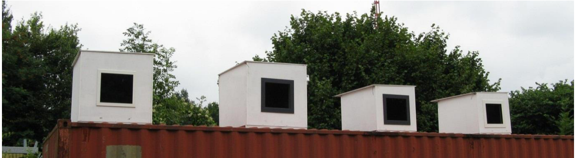
Fig. 1. Four insulated boxes containing concrete floors, with and without PCMs, as part of our experimental set-up at the University of Twente [29].
