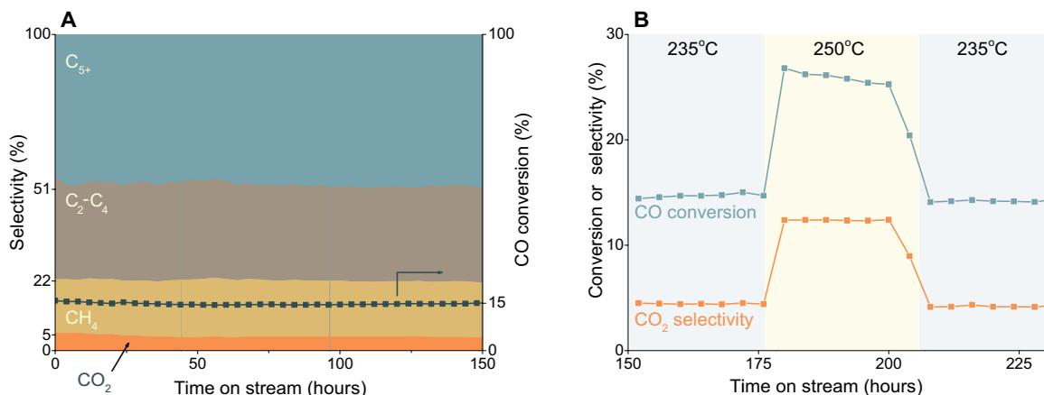
**Fig. 5. FT performance of the R-Fe catalyst as a function of time on stream.** (A) H<sub>2</sub>/CO = 1.5, 23 bar, 235°C, GHSV of 18,000 hour<sup>-1</sup>. (B) After 175-hour time on stream, the reaction temperature was increased to 250°C and kept there for 24 hours followed by a decrease to 235°C.
