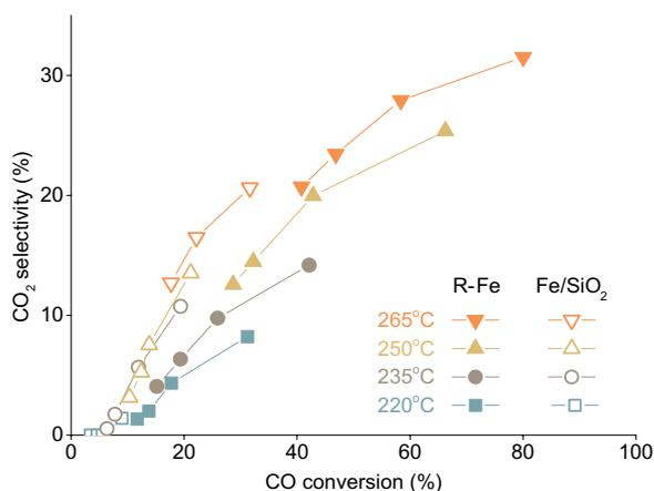
**Fig. 6.** CO<sub>2</sub> selectivity as a function of CO conversion on R-Fe (solid) and Fe/SiO<sub>2</sub> (open) catalysts at different temperatures. The CO conversion is varied by adjusting the flow rate at a constant H<sub>2</sub>/CO ratio.
