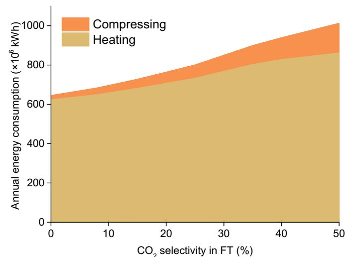
**Fig. 1. The influence of the CO<sub>2</sub> selectivity in the FT reaction on the annual (8000 hours per year) energy consumption of a 500 kton year<sup>-1</sup> liquid fuel production FT plant (including reactor, heater, compressor, and separator).**
