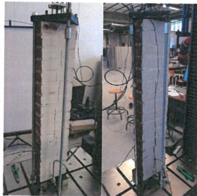
Figure 11: Marked hairline cracks during post-peak loading of the front (left) and back side (right).
