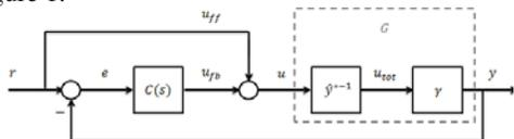
The proposed control approach relies on the availability of an accurate model  $\hat{\gamma}$  of the system  $\gamma$ , of which an (approximate) inverse  $\hat{\gamma}^{-1}$  exist. Thus, to allow for control-focused identification, only invertible model structures should be considered. For simplicity, this work limits itself to the Duhem model [1]; a nonlinear dynamic hysteresis model that is dependent on only 4 parameters. In [2] an approximate inverse of the Duhem model has been derived.
