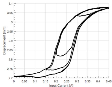
Although less suited for the Bouc-Wen model, the model-functions are adopted from [1], and thus are optimized for Shape Memory Alloy actuation. More research should be done on suitable invertible Bouc-Wen models.
