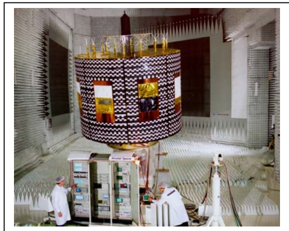
Figure 6. MSG Flightmodel Antenna Subsystem in the RF testrange (courtesy ThalesAleniaSpace Cannes -France).
