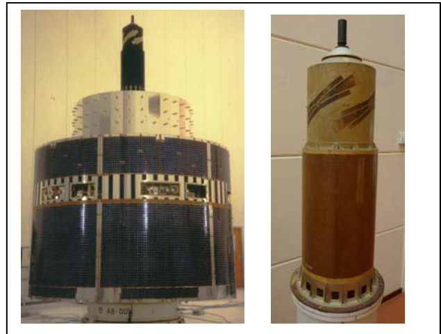
Figure 3. MOP Satellite with L-band EDA and antenna tower (left). The antenna tower (on the right) has a UHF Lindenblatt antenna and S-band quadrifilar helix. The lower compartment houses two slotted waveguide antennas.
