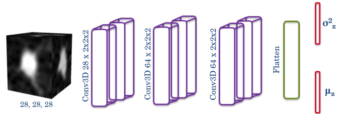
Figure 15: Trained 3D VAE architecture for Encoder
