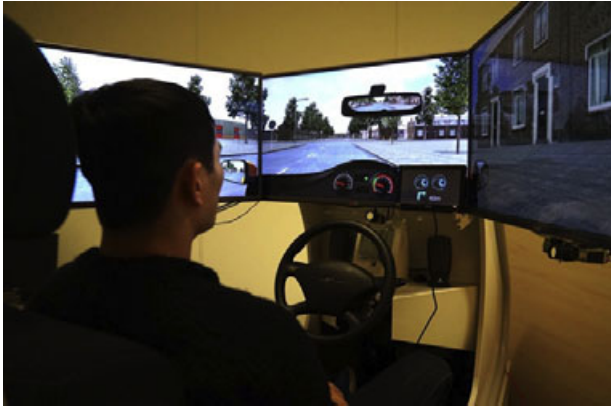
FIGURE 3 Snapshot of a participant in the driving simulator. The symbolic information and anthropomorphic representation are shown on the small screen at the lower right corner of the middle screen inside the driving simulator
