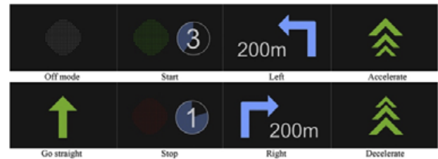
FIGURE 1 Contents of symbols. 'Start' and 'Stop' count backwards from 5 seconds to 0 (in the figure, snapshots are shown representing "still 3 seconds to go" and "still 1 second to go" for 'Start' and 'Stop' respectively). 'Left' and 'Right' count backwards from 200 meters to 0 with a step size of 50 meters. When the distance to the junction is less than 50 meters, the step size changes to 10 meters
