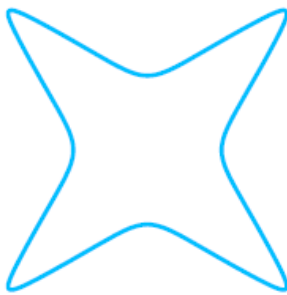
d) a; b = 1, m_1, m_2 = 4, n_1 = 10, n_2; n_3 = 30 and f[\theta] = 1, 0 \leq \theta \leq 2\pi
