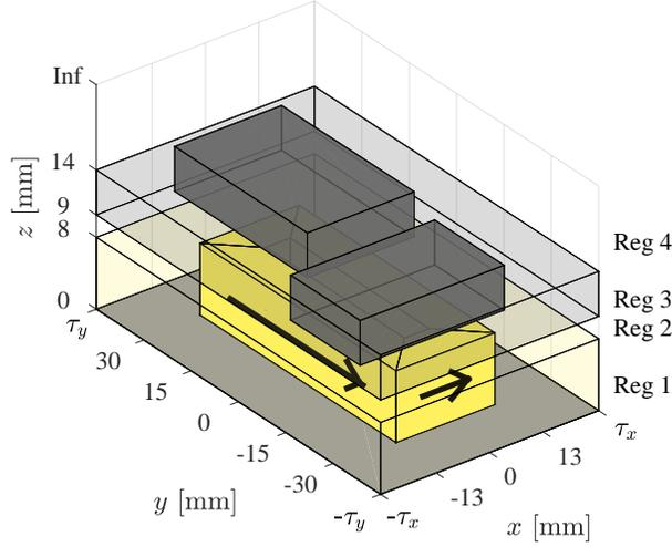
Fig. 1. Three-dimensional geometric model of two conducting plates (gray) placed above a time-varying current carrying coil (yellow).
