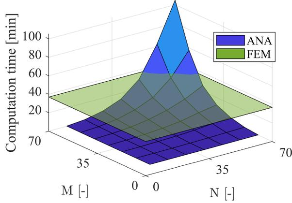
Fig. 9. Computation times of the compared methods.
