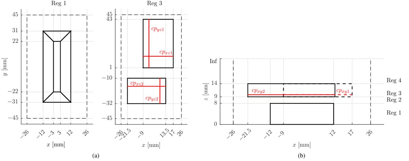
Fig. 3. Dimensions of the coil and plates in the modeled geometry: a) *xy*-view, b) *xz*-view.
