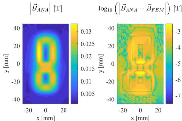
Fig. 6. Absolute value of the magnetic flux density on the  $xy$ -plane at  $z = 8.5$  mm. The result obtained with the semi-analytical model (ANA) is shown on the left side. On the right, the difference with the FEM result is depicted.
