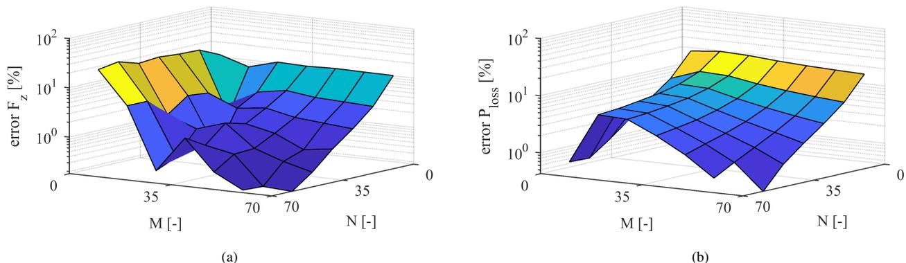
Fig. 4. Convergence plots as a function of the number of harmonics at a frequency of 100 Hz. The relative error with respect to the result at  $N = M = 70$  is calculated for each harmonic pair: a) convergence of the force in the  $z$ -direction, b) convergence of the power loss (in both conducting segments).
