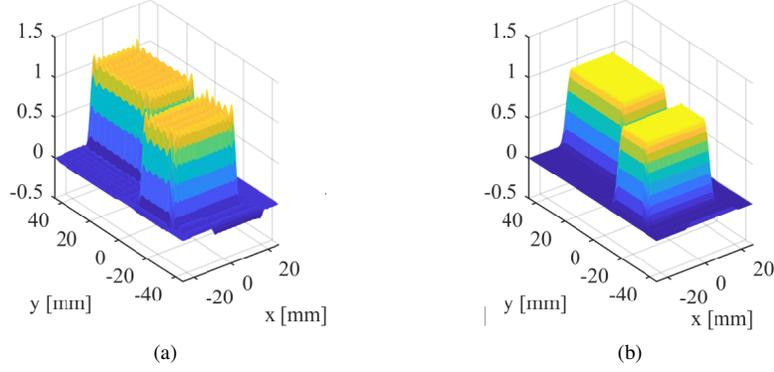
Fig. 2. Truncated Fourier series description of the conductivity in Region 3. a) Fourier description without Lanczos sigma factor multiplication. b) Fourier description with Lanczos sigma factor multiplication.
