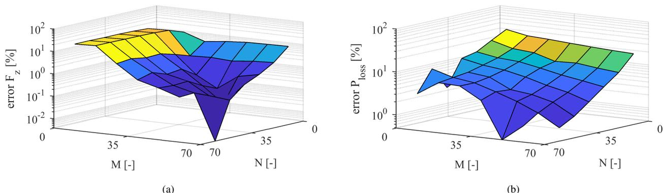
Fig. 5. Convergence plots as a function of the number of harmonics at a frequency of 10 kHz. The relative error with respect to the result at  $N = M = 70$  is calculated for each harmonic pair: a) convergence of the force in the  $z$ -direction, b) convergence of the power loss (in both conducting segments).
