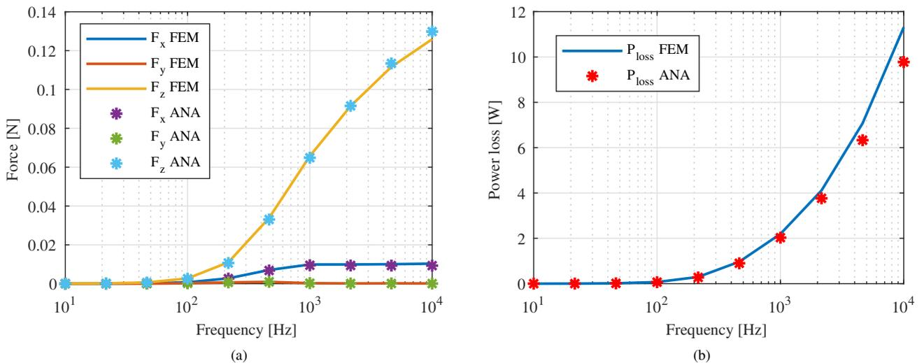
Fig. 8. a) Force components calculated with the developed semi-analytical (ANA) model and FEM. b) Power loss calculated with the developed semi-analytical (ANA) model and FEM.
