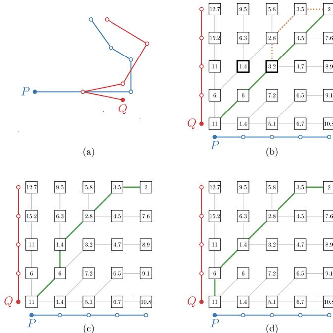
**Fig. 13.** Example illustrating that a preference order that prefers the diagonal parent over the two orthogonal ones may lead to incorrect results. (a) The input curves. (b) The tree constructed by the algorithm using the incorrect order. The orange dotted path proves that the matching described by the thick line is not locally correct. (c)–(d) The tree constructed by the algorithm when preferring the downwards and leftward neighbor respectively.
