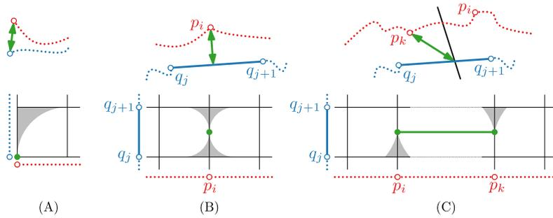
**Fig. 4.** Schematic illustration of the three critical events. Both the curves (top) and the free-space diagram (bottom) are illustrated. (A) Endpoints can be matched. (B) A passage between adjacent cells opens. (C) A passage opens between nonadjacent cells. The bisector is indicated with a black line.
