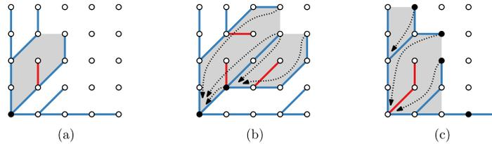
**Fig. 12.** (a) Face of tree (gray area) with its unique sink (solid dot). A red line represents a dead path. (b) Two adjacent faces with some shortcuts indicated. (c) Tree with three faces. Solid dots indicate growth nodes with a growth node as parent. These nodes are incident to at most one face. All shortcuts of these nodes are indicated.
