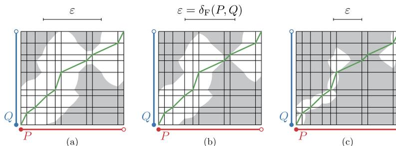
**Fig. 3.** Free-space diagrams for the curves of Fig. 1 with three different values of  $\varepsilon$ . The locally correct Fréchet matching is shown using a green path, crossing the diagram from bottom-left to top-right. (We refer the reader to the online article for colored versions of the figures in this article.)
