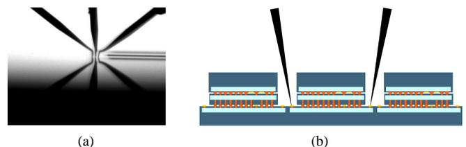
**Figure 5:** Wafer access challenges for post-bond stack test: die stacks (a) obstructing the contact view (here: top die is only 25  $\mu\text{m}$ ), and (b) the probe needle movement.
