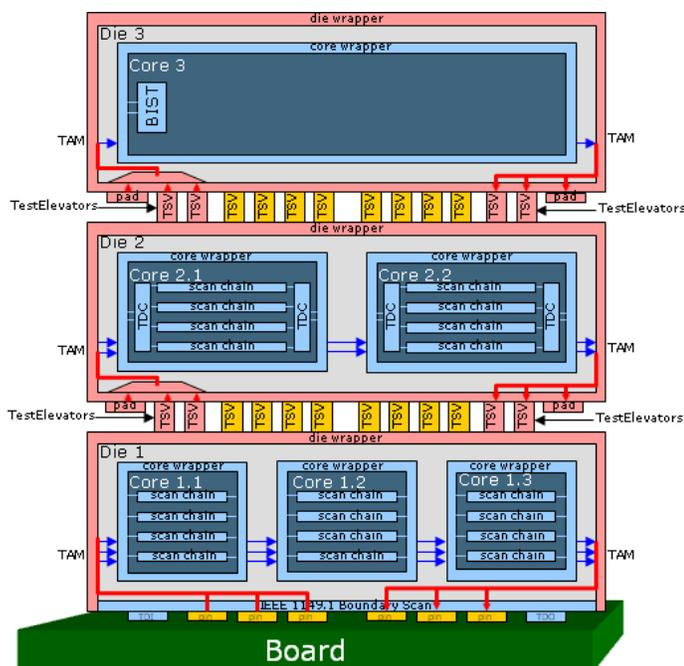
Figure 6: Overview of a 3D DfT architecture based on die-level wrappers.
