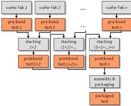
**Figure 2:** Overview of potential 3D test flows.
