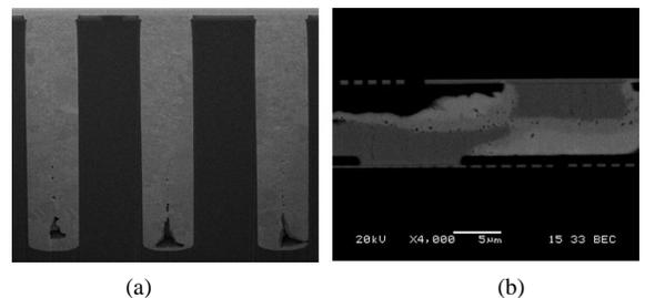
**Figure 3:** Examples of interconnect defects: (a) TSVs containing micro-voids, and (b) mis-aligned micro-bumps.
