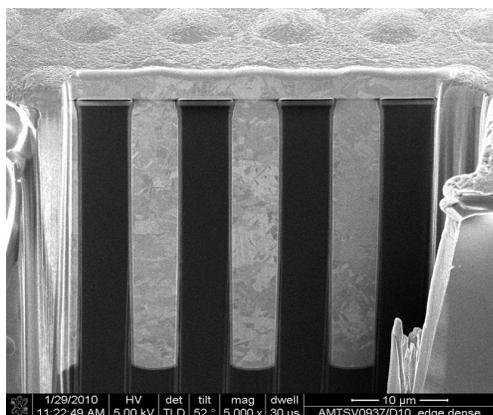
Figure 1: Cross-section photo of Through-Silicon Vias with aspect ratio 10:1.
