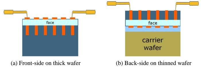
**Figure 4:** Pre-bond wafer probe options on (a) a thick or (b) a thinned-down die.
