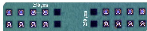
Fig. 4: Micrograph taken from the interposer's backside, the apertures of the PD/VCSEL can be seen through OTSVs.
