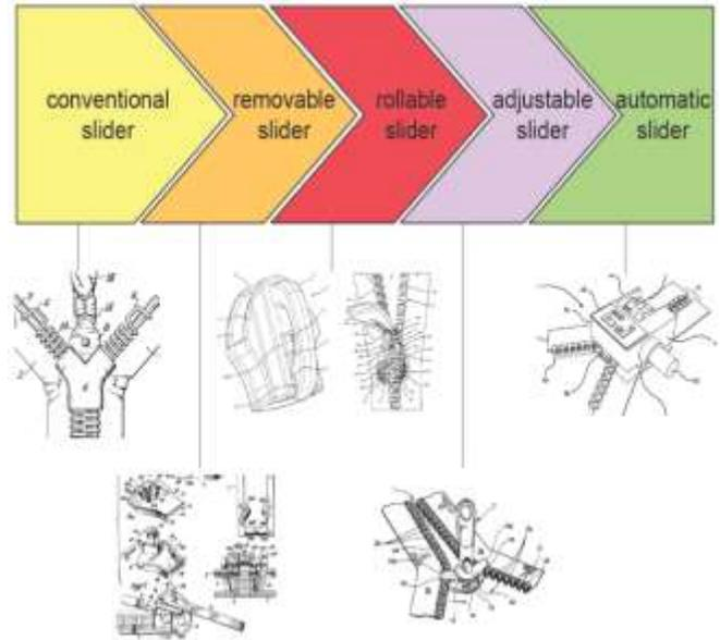
**Figure 9. The evolution of the slider** [10], [13], [31], [36], [38], [39]
