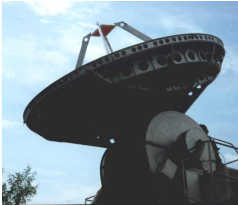
Fig. 2. Large antenna with polarization grid in focal area
