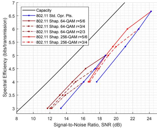
Fig. 11. Packet error probability =  $10^{-2}$ . For each point, 4 different simulations are completed, and for each of them at least 200 packet errors are collected.  $r=\{2/3, 3/4, 5/6\}$  with 64-QAM, and  $r=\{3/4, 5/6\}$  with 256-QAM are allowed combinations in 802.11. The others are simulated to provide references. Note that there is a  $10 \log_{10}(52/64) \approx -0.9$  dB difference between the observed and the actual SNR values since 12 out of 64 subcarriers are empty in [6].
