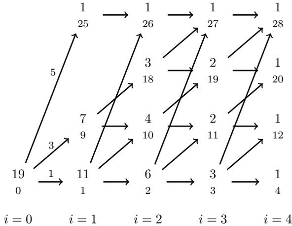
Fig. 2. Enumerative shaping trellis for  $n = 4$  and  $E_{max} = 28$ .
