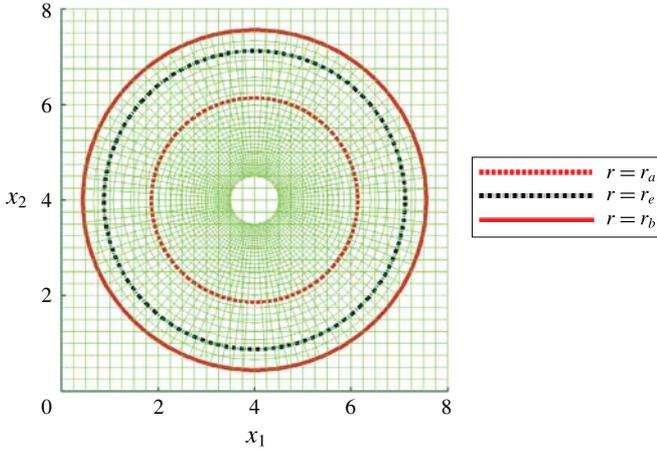
FIGURE 1. (Colour online) Illustration of the concentric spheres,  $r = r_a$ ,  $r = r_e$  (defined in § 2.4) and  $r = r_b$ , drawn on the overlapping grids used to mesh the region around one of the 64 particles in simulation L128 introduced in § 3. Part of the plane  $x_3 = 4$  is shown.
