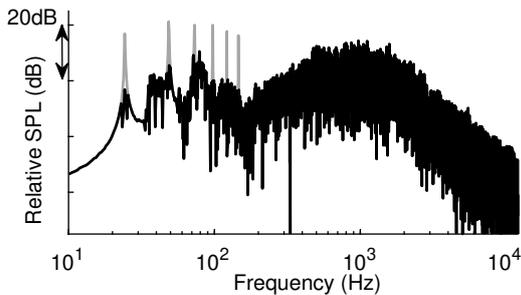
Figure 1: Spectrum of a dry car signal (70 km/h) with (grey) and without (black) tonal components used in the auralizations presented in this work.
