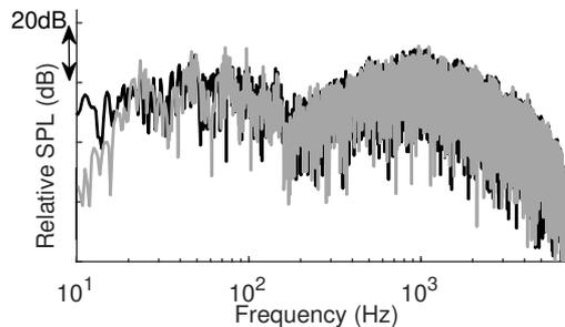
Figure 6: Spectrum of auralization signals 70TA2 (reference) (black line) and 70TA8 (grey line). The spectrum was computed by taking the FFT of the total duration (2.9 s) of the test signals. See Table 1 for notations. SPL stands for sound pressure level.
