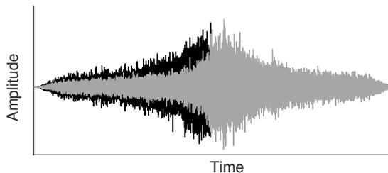
Figure 5: Final auralization signals for left (black) and right (grey) ears. These signals were created by adding the signal blocks shown in Figure 4 (b) (which has to be done for the left and right signal separately).
