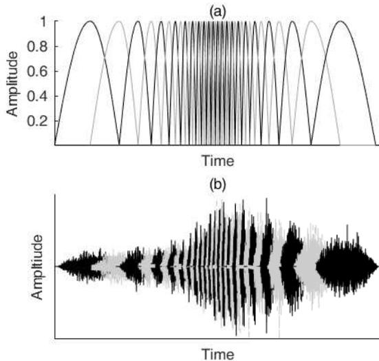
Figure 4: (a) Window functions according to equation (2) that were multiplied by the dry car signal blocks. (b) Overlapping windowed car signals blocks convolved with their corresponding BIR.
