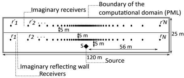
Figure 2: Schematic layout of the 2D PSTD domain where  $S$  is the source,  $r_n$  are the receivers used to simulate the direct sound and  $r'_n$  are the receivers that were used to synthesize the 1st order specular reflection.
