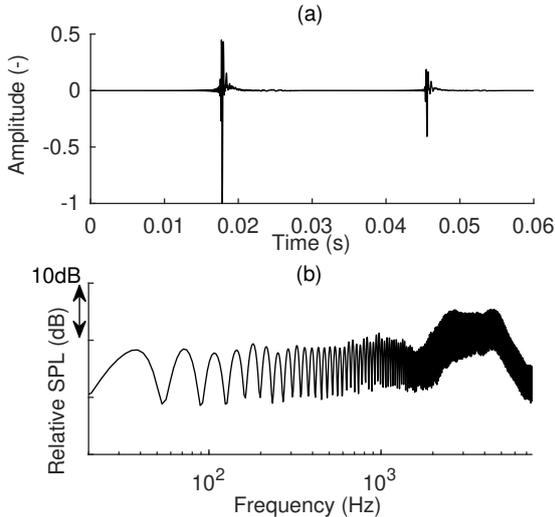
Figure 3: (a) Post-processed and normalized right ear BIR for the receiver at 35° and 6.1 m from the source including the corresponding mirrored image (see Figure 2) and (b) its frequency response.
