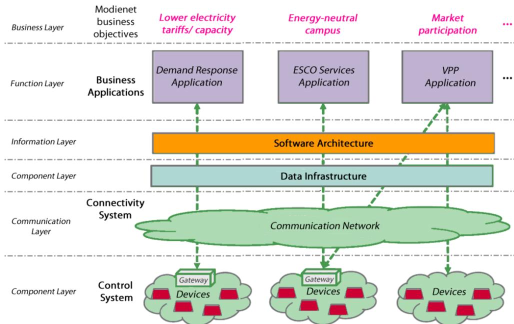
Fig. 9. The Modienet ICT System described in terms of SGAM (Adapted from [26])
