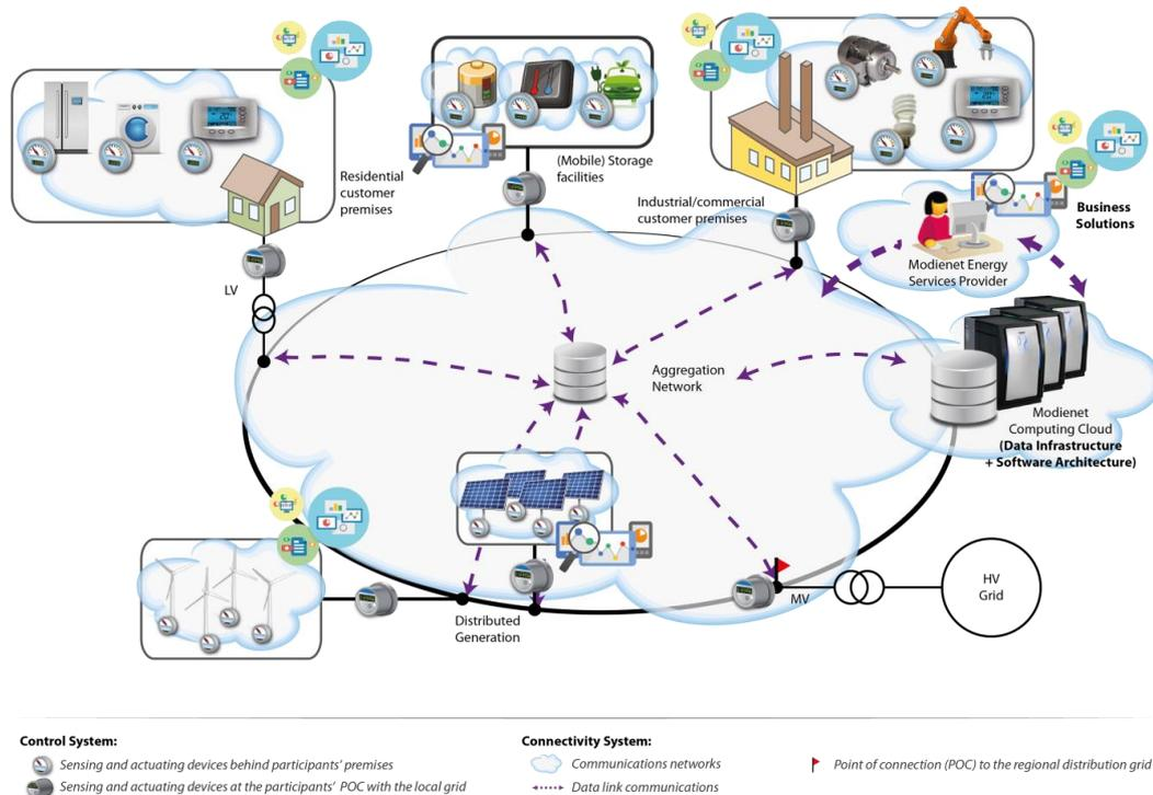
Fig. 19. The Modienet ICT platform concept (Adapted from [41])
