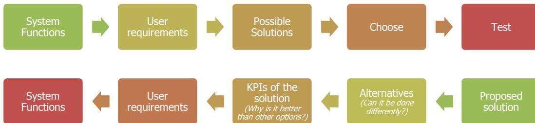
Fig. 7. Comparison of the "Reverse" SE method (bottom) with the original methodology (top)
