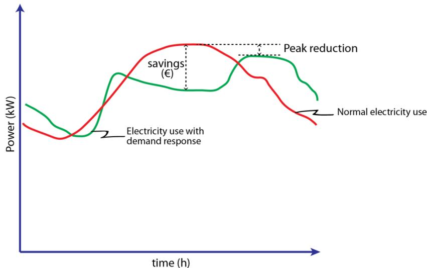
Fig. 21. Schematic representation of a peak-shifting demand-response mechanism
