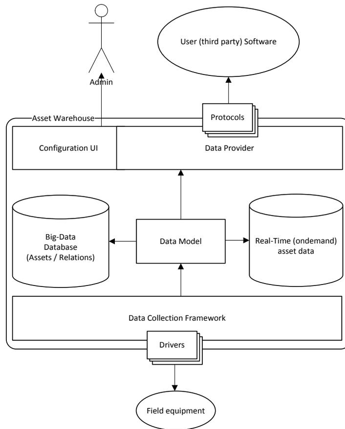
Fig. 18. System architecture of the data warehouse
