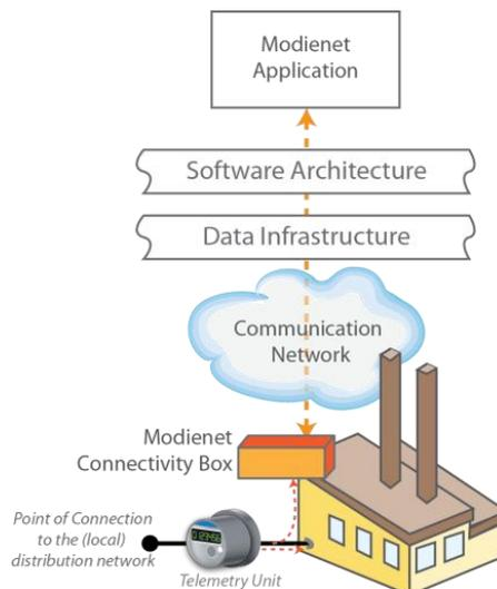
Fig. 14. Extracting telemetry data for use in the Modienet Application
