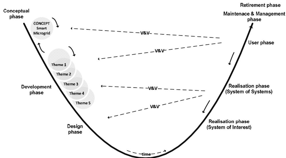
Fig. 5. The SE iterative development method for Smart Microgrids [23]
