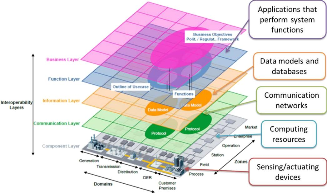
Fig. 8. ICT systems components abound in all layers of the SGAM. (Adapted from [19])
