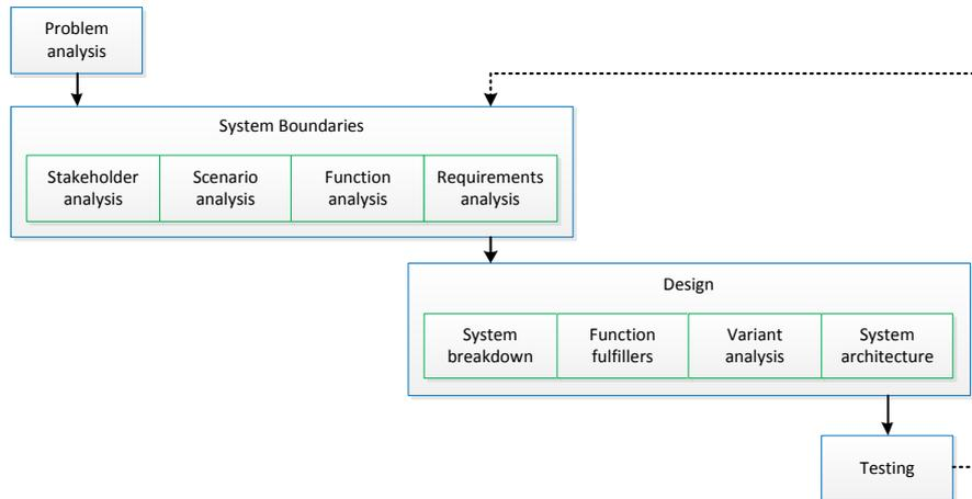
Fig. 4. Schematic of the Systems Engineering design process (Adapted from [24])
