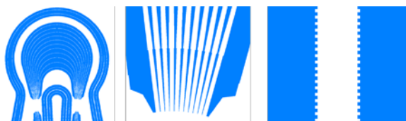
Figure 1: Examples of geometries in PICs: Bends (Left), Tapers (Middle), Subwavelength modulation features (Right).
