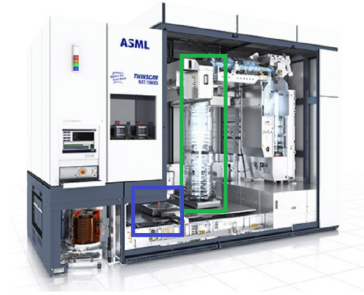
Figure 1.2: The TWINSKAN System. In blue the measurement side and green the exposure side.
