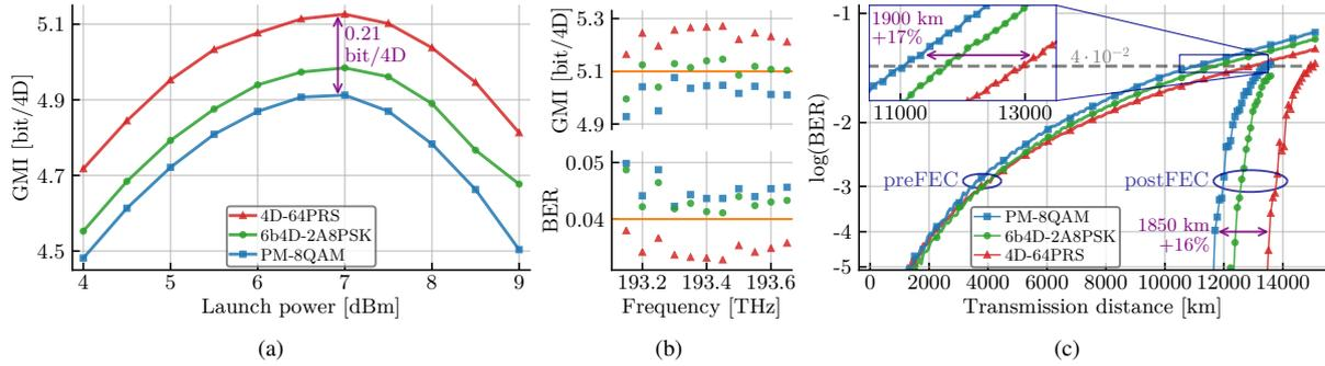
Fig. 3: Experimental results using a hybrid of EDFA and Raman amplification. **(a)** Average GMI per channel versus total launch power after 12,530 km. **(b)** Per-channel performance versus BERs (top) and GMIs (bottom) measured for all 11 channels individually after 11,700 km showing BERs below the FEC threshold  $4 \cdot 10^{-2}$  [2] (top) and GMIs above 5.1 bit/4D [8]. **(c)** BER versus transmission distance for the center channel at launch power of 6.5 dBm.
