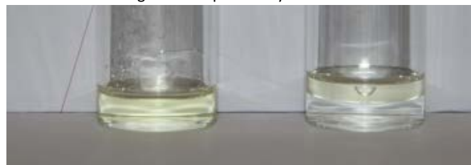
Figure 2: (left) pure DES DecA:N 4444 -Cl (2:1) and (right) DecA:N 4444 -Cl (2:1) after mixing with water.
