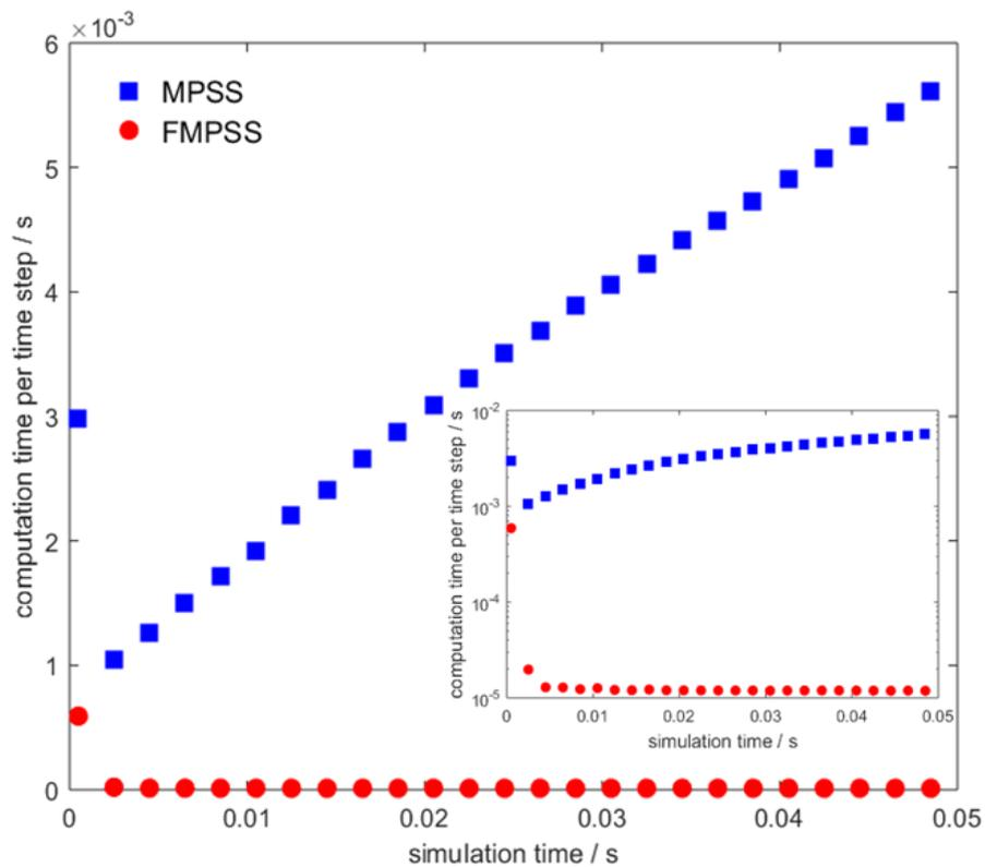
**Figure 4.** Comparison of computation time using MPSS and FMPSS using parameters listed in Table 1. The results correspond to  $M = 40$ . Inset showing semi-logarithmic plot of computation time. Approximately three orders of magnitude speed improvement is achieved by the FMPSS method.
