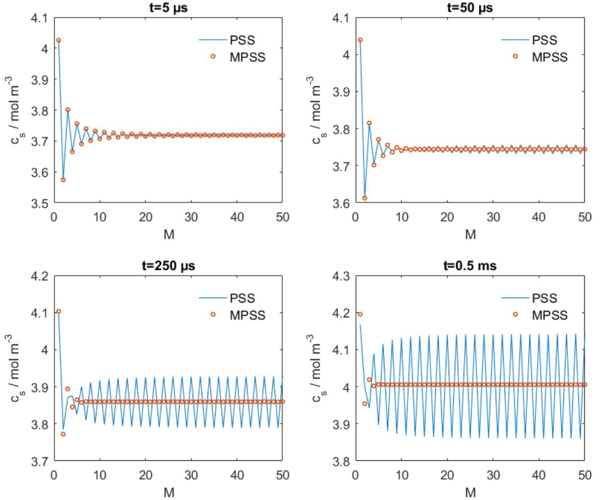
**Figure 3.** Convergence of the MPSS and PSS methods as a function of  $M$ , the number of terms in summation. PSS solutions become oscillatory as time increases while the MPSS method gives uniform convergent solutions at all times.
