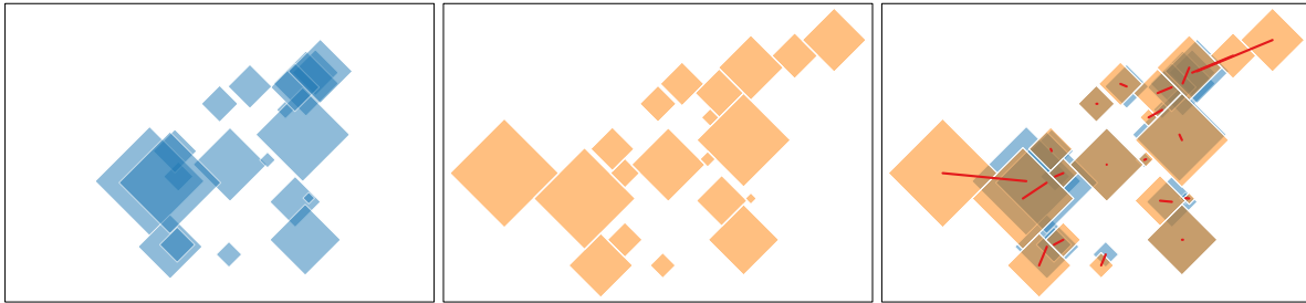
Figure 1: Left: example input of overlapping diamonds. Middle: output of the suggested linear program, having minimal displacement and maintaining the orthogonal order. Right: overlay visualizing the displacement of each diamond.
