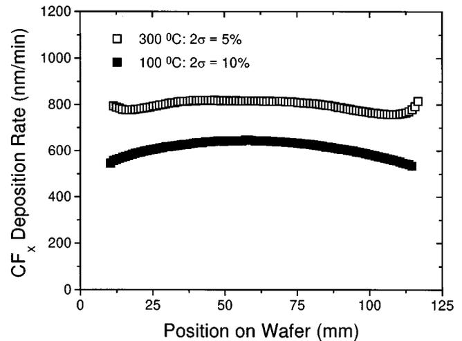
FIG. 14. The fluorocarbon deposition rate profiles as a function of position on the wafer obtained in a  $C_3F_6/H_2$  (40 sccm/15 sccm) discharge at 1400 W inductive power and 6 mTorr operating pressure. The open symbols correspond to a condition where the reactor wall temperature is around 300 °C. For the solid symbols the reactor wall temperature is around 100 °C. The fluorocarbon deposition uniformity is 10% ( $2\sigma$ ) at 100 °C and 5% ( $2\sigma$ ) at 300 °C.
