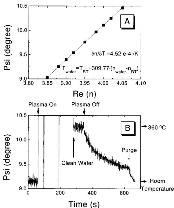
FIG. 6. (A) Simulated correlation between the ellipsometric angle  $\Psi$  measured on a crystalline silicon wafer and the real part of the refractive index of the silicon. (B) Ellipsometric angle  $\Psi$  measured as a function of time on a non-cooled crystalline silicon wafer in a  $C_3F_6$  plasma at 1400 W inductive power and 6 mTorr operating pressure.
