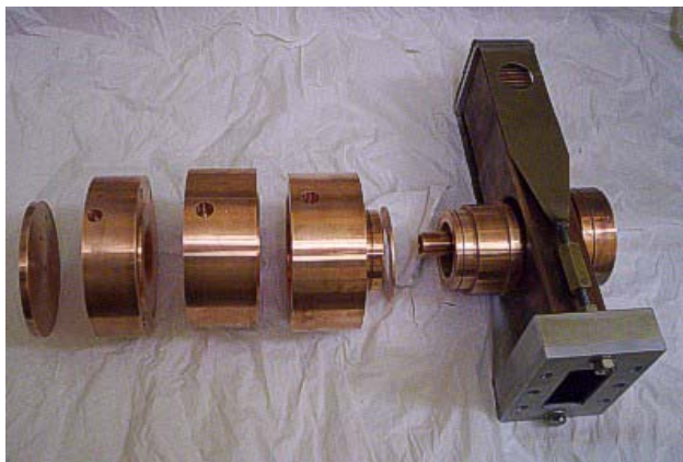
Figure 3: Cavity cells and input coupler prior to brazing.
