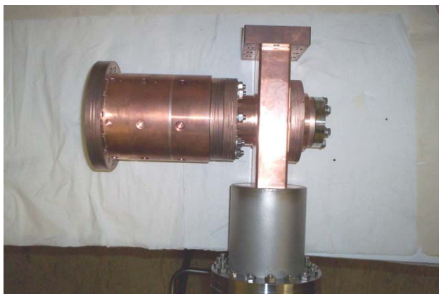
Figure 7: The completed ALPHA-X photo-injector.
