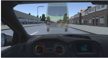
Figure 1: Concept of translucent road objects: Using large-scale windshield displays and video streams (e.g., from a lead vehicle), the objects around the driver can be made translucent. The idea is that this supports the driver in anticipating for example pedestrians who plan to cross the road.
