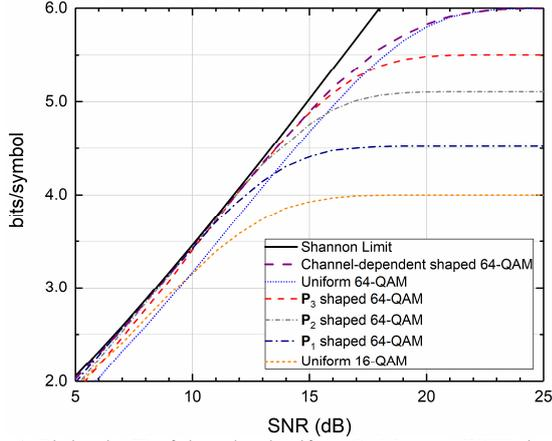
Fig. 1. Bit-level AIR of shaped and uniform QAM over AWGN channel.
