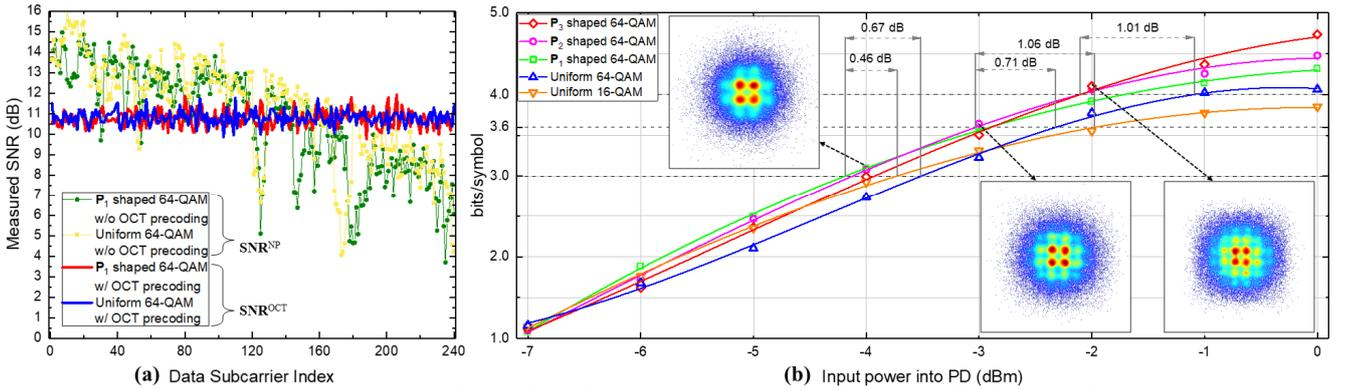
Fig. 4. (a) Measured SNR vs. data subcarrier at -3 dBm of PD input power. (b) Measured AIR vs. PD input power with OCT precoding.
