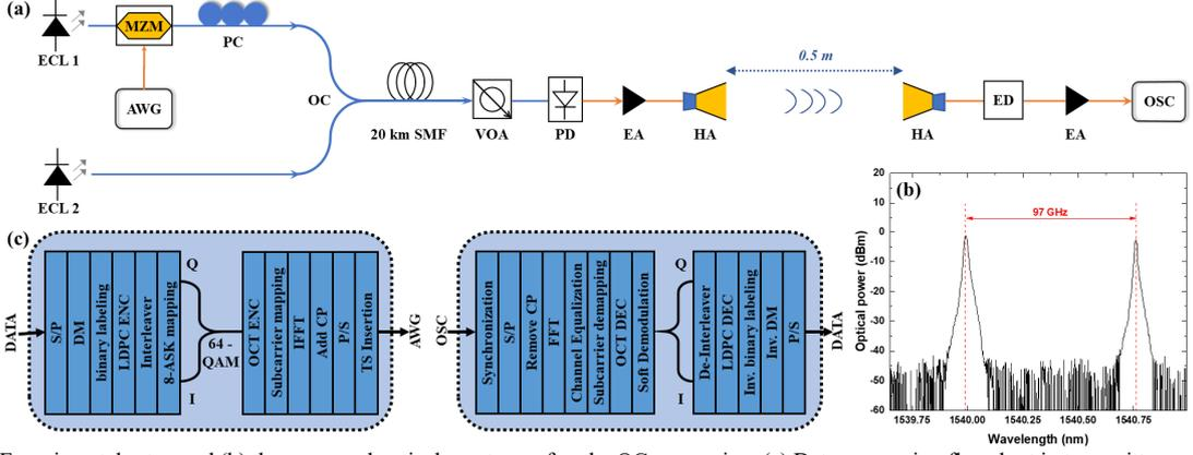
Fig. 2. (a) Experimental setup and (b) the measured optical spectrum after the OC processing. (c) Data-processing flowchart in transmitter and receiver.
