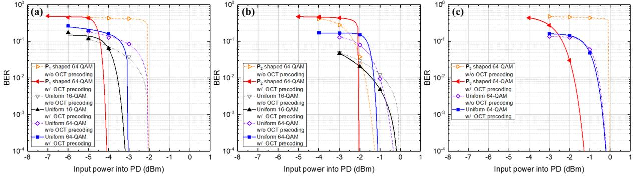
Fig. 3. BER fitting curve vs. input power into PD of shaped and uniform scheme.  $R_{UNI} = R_{PAS} =$  (a) 3.0; (b) 3.6; (c) 4.0 (bits/symbol).
