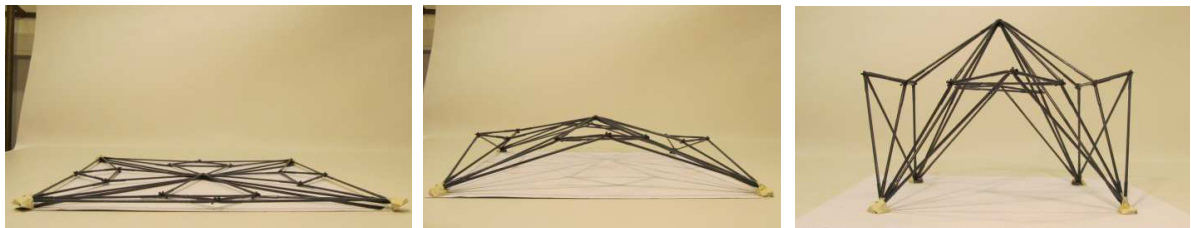
Figure 3. Hinged connected bar model, in different folding states
