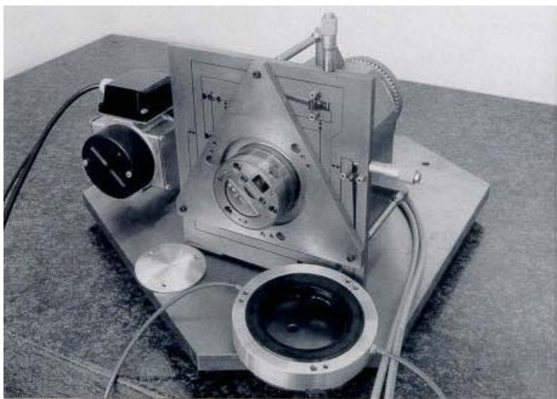
Figure 6: Photograph of RLS 2 test rig for film thickness measurements (the test seal is removed). See text.
