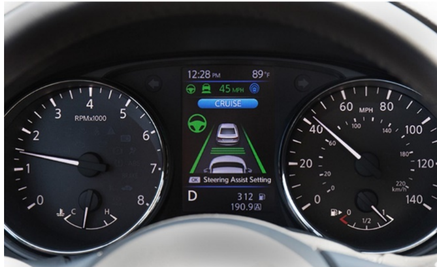
Figure 1-2: An illustration of a HMI where the driver is informed about lateral assist status. The green lines indicate that the lane markers are detected and the system can be activated [3].
