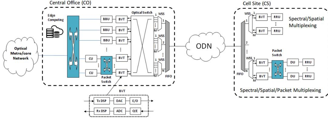
Figure 2: DRoF signal distribution scheme. BBU: Baseband unit; BVT: bandwidth/bitrade variable transceiver; CU: central unit; DU: distributed unit; FIFO: Fan in/out device; RRU: remote radio unit; WSS: wavelength selective switch. Insets show a simplified BVT scheme and the corresponding DSP blocks.
