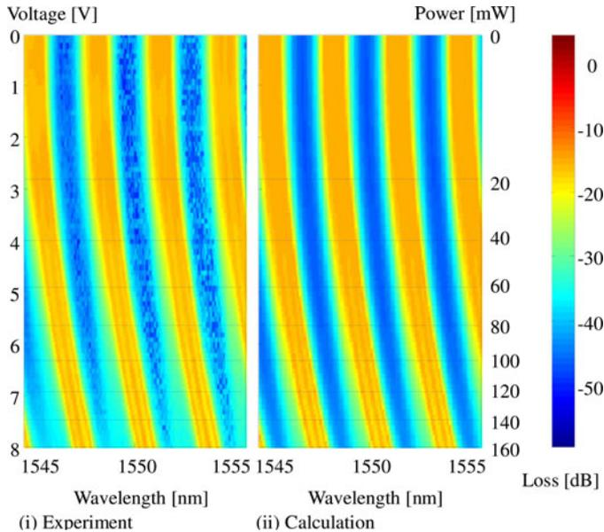
Fig. 4. Thermal tuning of the switch element connecting input 1 to output 1. Experimentally measured optical transfer functions (left) and calculated transfer functions using the transfer matrix model (right).
