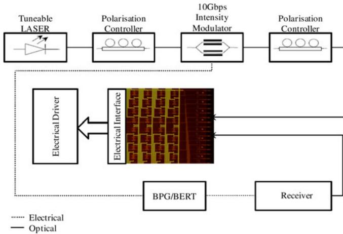
Fig. 8. Schematic of the experimental setup used for 10-Gb/s data routing.
