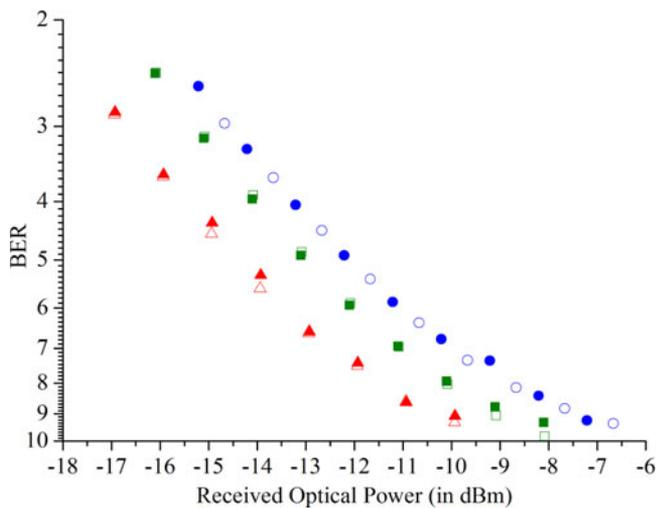
Fig. 10. Bit-error Rate curves of the measured paths at 40 Gb/s using a  $2^{31}-1$  PRBS sequence. The solid and open symbols represent the routed and back to back measurements for path 1 to 1 (■), 2 to 2 (▲) and 3 to 3 (●) respectively.TABLE V
