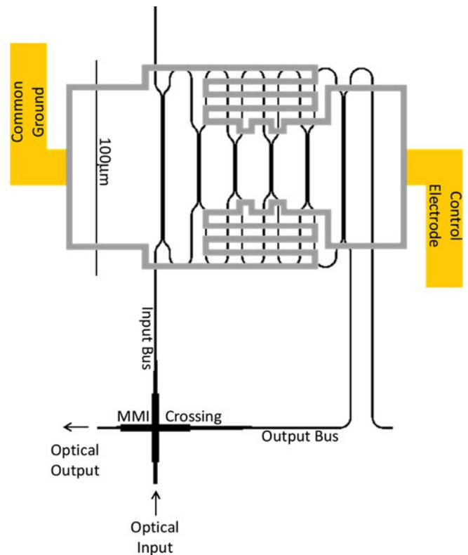
Fig. 2. Mask details for one switch element. The optical waveguides are shown in black. The narrow Ti/Pt micro-heater features are shown in grey, and the wider gold on-chip wiring is shown in orange.
