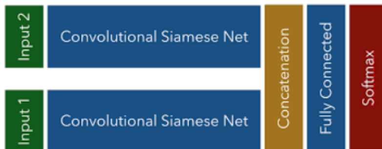
Figure 2.3: Architecture of a Siamese Convolutional Neural Network
