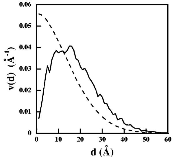
FIG. 9. Solid line: vacancy distribution  $v(d)$  calculated with TRIM for 1 keV Ar<sup>+</sup> ions incident at 45°. The dashed line corresponds to the steady-state vacancy distribution when the movement of the surface is included.
