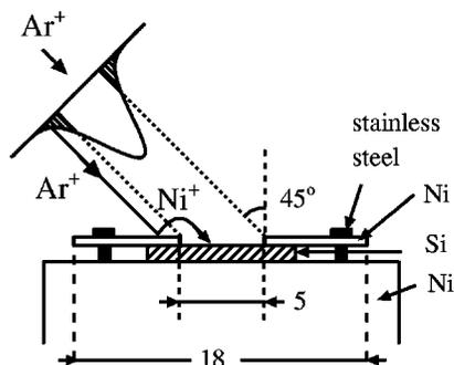
FIG. 1. Sample holder. The various sizes of the components are indicated in mm. As the  $\text{Ar}^+$  ion beam partly hits the nickel retainer plate,  $\text{Ni}^+$  can be sputtered and deposited on the Si sample (hatched) by a bias voltage of  $-100$  V.
