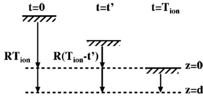
FIG. 8. Schematic view of the surface position during ion-enhanced etching, as used for the calculation of the steady-state vacancy distribution during ion-assisted etching from  $t=0$  to  $t=T_{\text{ion}}$ . The depth  $d$  is defined with respect to the surface position at  $t=T_{\text{ion}}$  when the etching is stopped.
