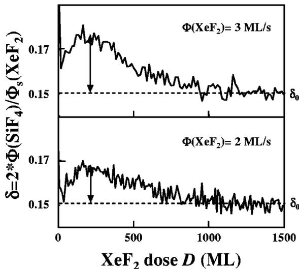
FIG. 3. Influence of the  $\text{XeF}_2$  flux on the enhancement of the production coefficient. The horizontal scale is the total dose of  $\text{XeF}_2$  after the ions have been switched off. Measurements are shown for  $\text{XeF}_2$  fluxes of 2 and 3 ML/s.
