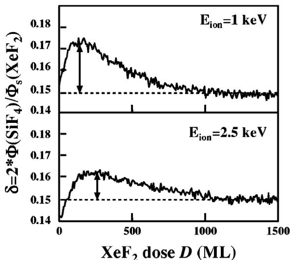
FIG. 6. Influence of the ion energy on the enhancement. The average response of three measurements is shown for 1 and 2.5 keV  $\text{Ar}^+$  ions after the Si is bombarded with a  $6 \mu\text{A}$  ion current for 60 s.
