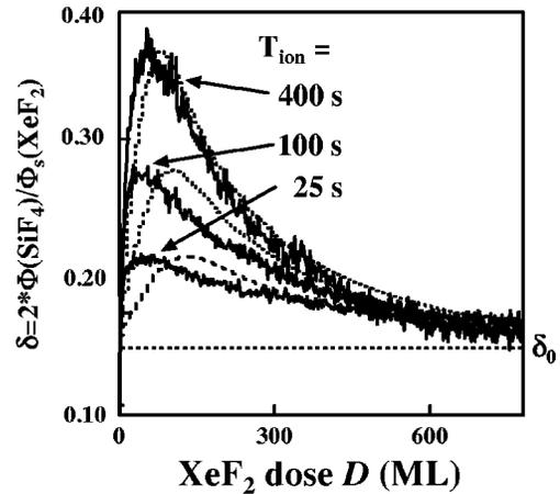
FIG. 11. Measurements (solid curves) and simulation (dotted curves) for the temporary enhancement due to tungsten contamination. The parameter  $\alpha$ , determining the maximum enhancement, is manually adjusted to compensate for the saturation of the maximum enhancement as a function of  $T_{\text{ion}}$ .
