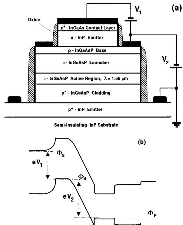
FIG. 1. Schematic (a) cross section and (b) energy band diagram of the proposed three-terminal laser structure, using InGaAsP, lattice matched to InP, material system. Both  $i$  launcher and  $p$  claddings are eventually graded layers, with band gap narrowing towards the active region.  $\Phi_N$ ,  $\Phi_P$ , and  $\Phi_B$  are the Fermi levels in  $N$ ,  $P$  emitters, and base, respectively.
