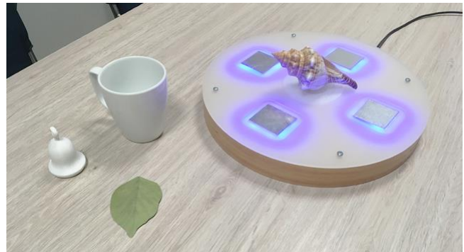
Figure 1. Placing the everyday object (e.g. seashell) on the dementia soundboard triggered the corresponding soundscape (e.g. beach). By touching the surrounding touchpads, each layer (e.g. beach_children) could be activated or deactivated.
