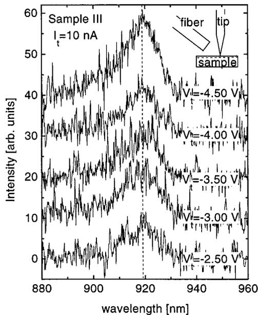
FIG. 1. STL signal from sample III at various  $V_t$  and  $I_t = 10$  nA. The integration time is 10 min. The insert schematically depicts the setup which is operated in ambient.
