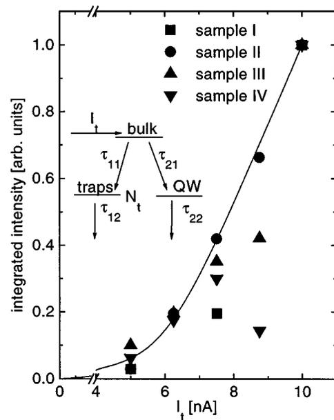
FIG. 2. Integrated STL intensity (normalized) vs  $I_t$  at  $V_t = -3.5$  V. The line is calculated from a three-level rate-equation model. Insert: Illustration of the rate-equation model.  $N_t$  is the number of available traps, the  $t_{ij}$  are relaxation times.
