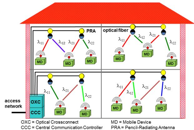
Fig. 1 Indoor OWC system using steered IR beams
