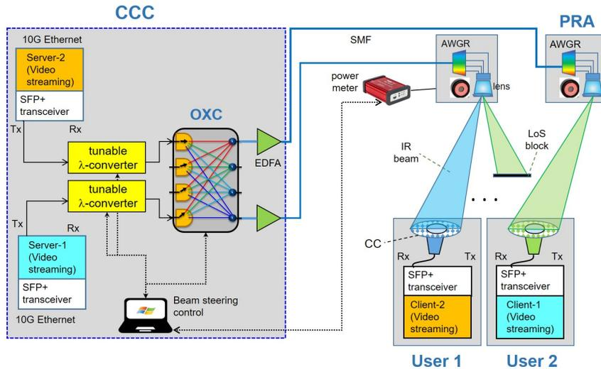
Fig. 5 Laboratory system demonstrator
