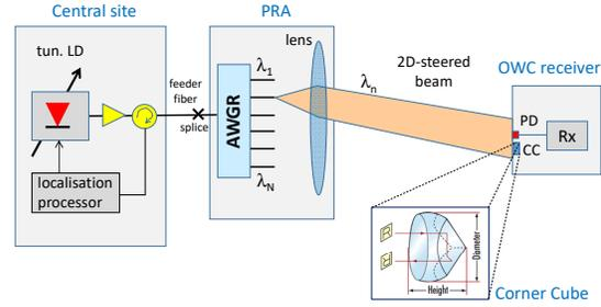
Fig. 3 Passive localization at user device by optical retroreflector
