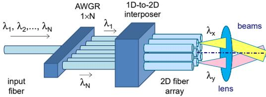
Fig. 2 AWGR-based 2D passive beam steerer
