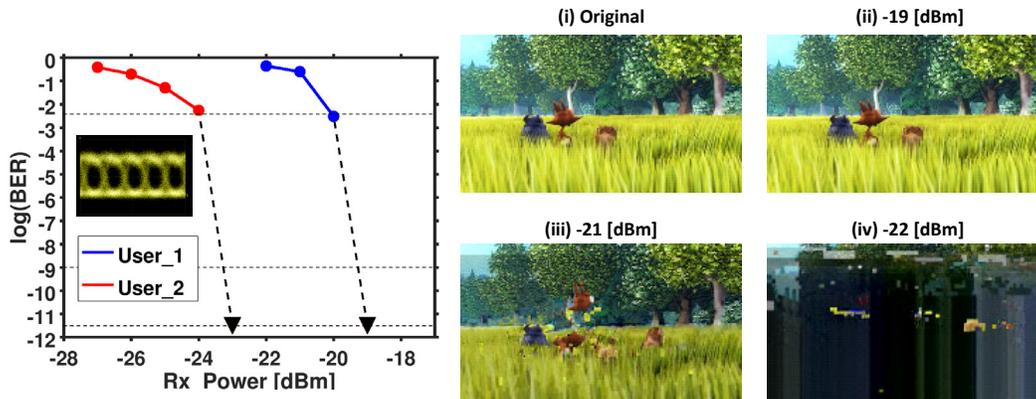
Fig. 3. BER performance of the real-time video signals. Lower triangle: minimum system BER at the corresponding Rx power.. Insets: the image quality of the corresponding receiving power.
