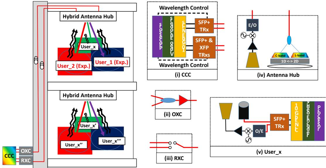
**Fig. 1.** AWG based 2-D PRA OWC system. Insets: the corresponding experimental unit setup. CCC: central communication controller; OXC: optical cross-connect; RXC: radio cross-connect; Exp.: used in experiment. NIC: network interface card.
