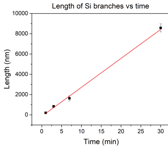
Figure 4.3 – A time series performed at 650 °C in which the length of the branches is measured. All the branches are grown with disilane on a Si shell, with a flow of 0.85 sccm. The growth rate seems to be constant at around 280\pm 10 nm per minute. Also, there is no evidence for an incubation time, indicating that the nucleation starts almost immediately after the flow with precursor gasses is opened.
